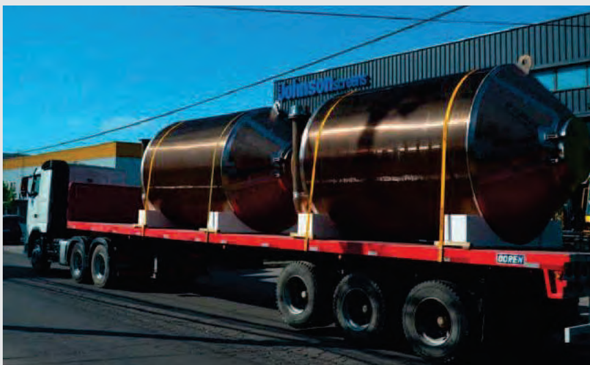
Transport of JOHNSON SCREENS® Passive Screens to the Santa Maria Power Plant at a Site in Chile
